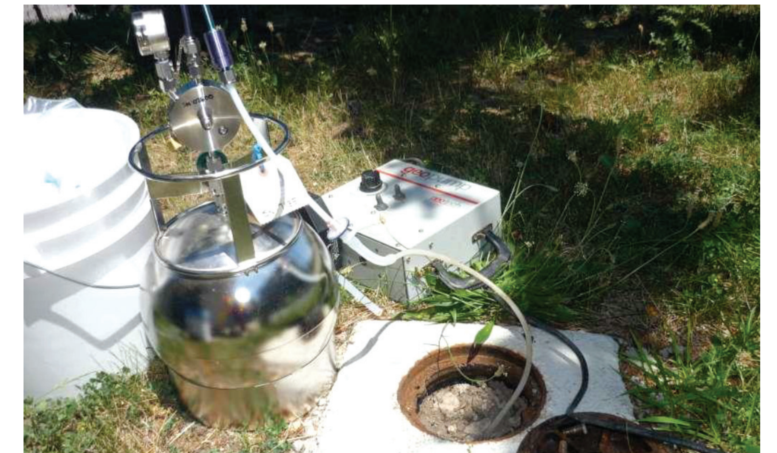
Sampling of a Source Area or Near-Slab Soil Vapor Well
