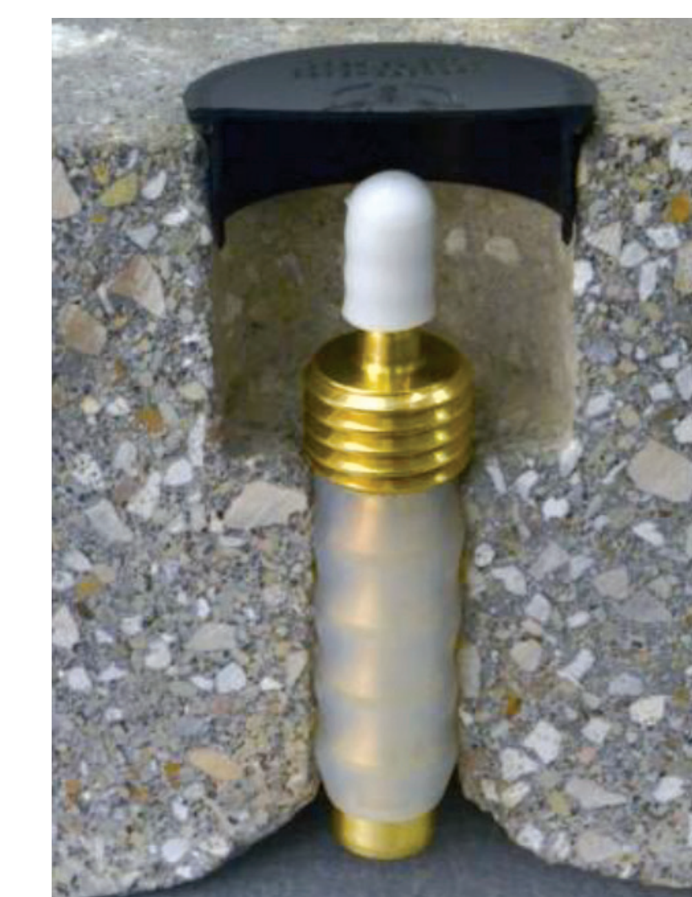
Sub-Slab Soil Vapor Pin
